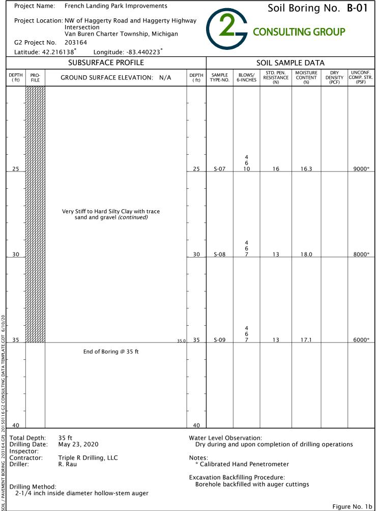
203164.GPI SOIL / PAVEMENT BORING
