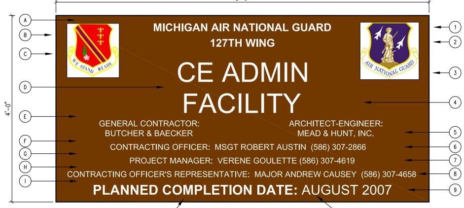
4'0" X 8'-0" SHEET OF  $\underline{J}$  " GRADE AC EXTERIOR PLYWOOD. - PAINT ALL SIDES ONE COAT PRIMER AND TWO COATS GLOSS EXTERIOR ENAMEL
