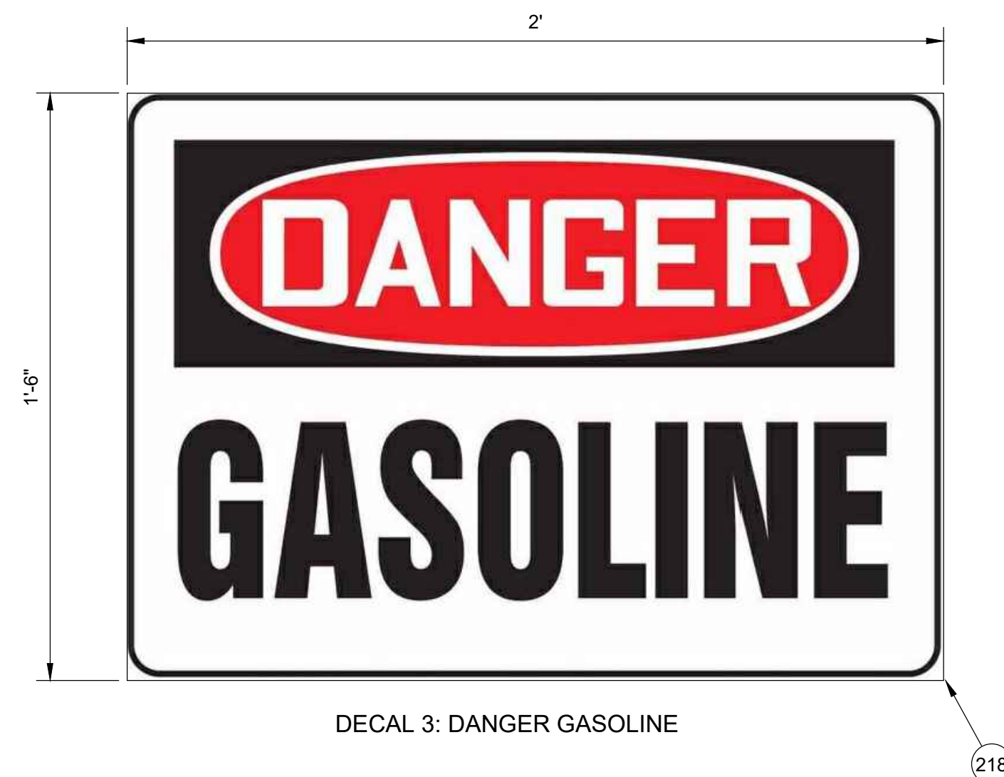
C GASOLINE AST SIGNAGE/DECALS SCALE: 3" = 1'-0"
